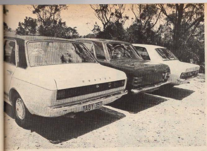
Cortina has the highest rear deck. Both Torana and Cortina have boot locks on the door, Hillman has it mounted on rear panel. Hillman is only one without wrap-around tail lights.
